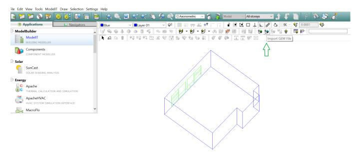
Click the *'import'* button, locate the folder where the geometry is saved, and open the *'GEM files.gem'* file as shown below (Shown here for the S1500 e-stack unit):
