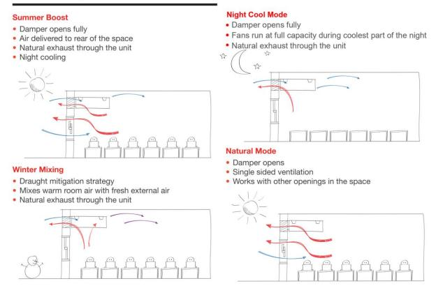
The NVHR system is not a heat exchanger, and therefore cannot be modelled as a mechanical system with heat recovery. The system saves energy by bringing air into the space and mixing it with the room air to reduce cold draughts.
