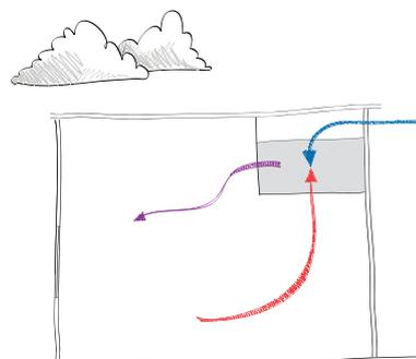
At the same time the hot, polluted air leaves the room via the second high level window that is opened and closed by the F-Series controller.
