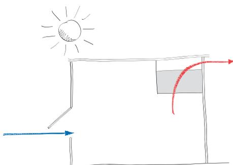
As the Breathing Buildings e-stack system generates its own natural and, if required, assisted upwards displacement of air, ventilation is assured and occupants are well ventilated even on hot, wind-free days.
