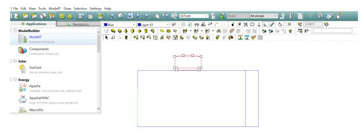
The e-stack unit is now at the correct height, but as can be seen from a plan view, its position is still not quite correct. In the plan view use the same 'move selection' set button to drag the e-stack unit to its correct position.
